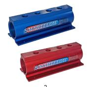
PCS Company offers Smartflow® 3/4" Aluminum Manifolds which are constructed from unique extruded aluminum, machined pre-cisely and then anodized for corrosion resistance. These manifolds are standardized in both red and blue to denote supply and return lines. Choose from a wide selection of standard Aluminum Mani-folds or contact PCS for a custom manifold. The 3/4" manifolds have pre-drilled mounting holes and supplied with bolts for ease of installation.
